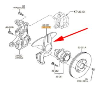
c. Rear backing plates/dirt shields may be removed.
